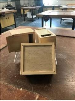
The year 8 Woodwork class has been working on making Treasure Boxes. To make this, the students drew up designs with their measurements, marked and cut their pieces and then cut rebate joins into the wood. Chiselling rebate joins is a tricky skill and the students have done very well at this.
